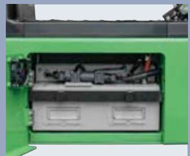
Lithium battery pack
