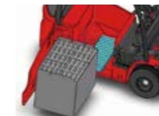
Battery side roll out by roller (Opt.)
